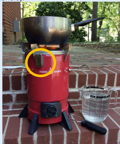
Figure 1: Mimi Moto improved cook stove with stove use monitor (SUM) (in yellow circle)
